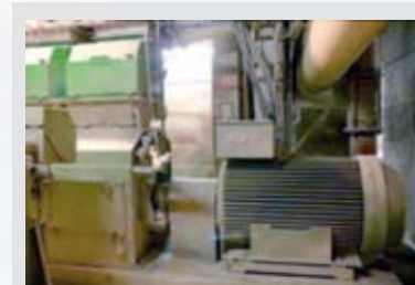
Original motor Frame size 355 mm 2-4P / 220 kW / 1750 kg
