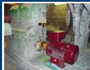
DYNEO solution Frame size 280 mm 3000 min -1 / 220 kW / 426 kg
