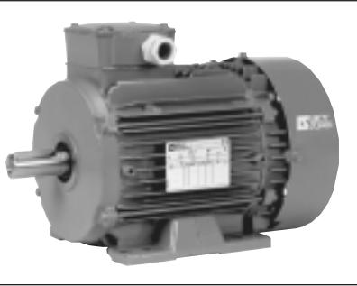
**3-phase brake induction motors, LS series,** failsafe with field deviator (without electro-magnet) power rating 0.18 to 0.55 kW, frame size 71 mm, 4, 6-pole ; 230/400 V, 50 Hz.
