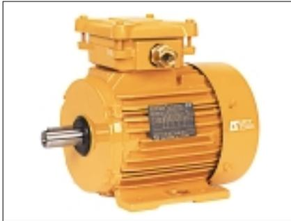
– **3-phase TEFV induction motors, FLSPX series with cast iron housing**, conforming to IEC 34, 72, EN 50281, power **0.18 to 400 kW**, frame size 80 to 355 mm.
